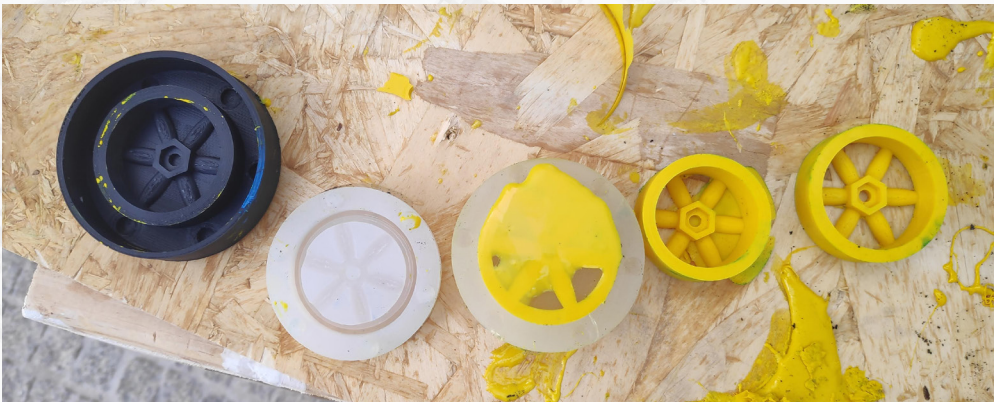
The rims are created with resin in silicone molds.
