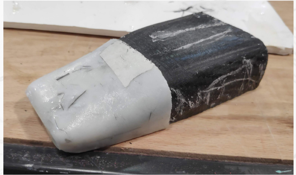
The bodywork is created from carbon fiber, with the molds being 3D printed.
