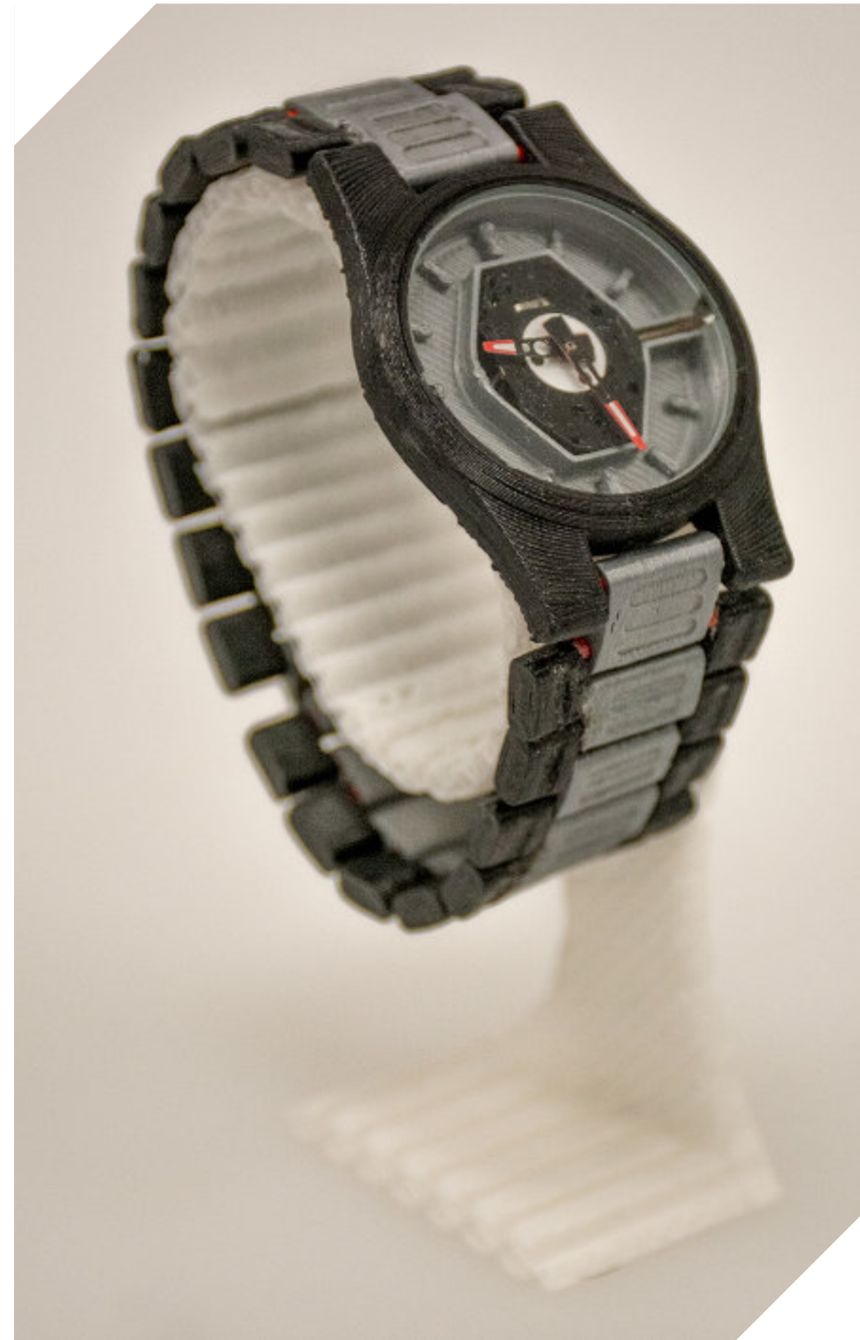
3D printed watch re-purposing an old watch mechanism and glass
