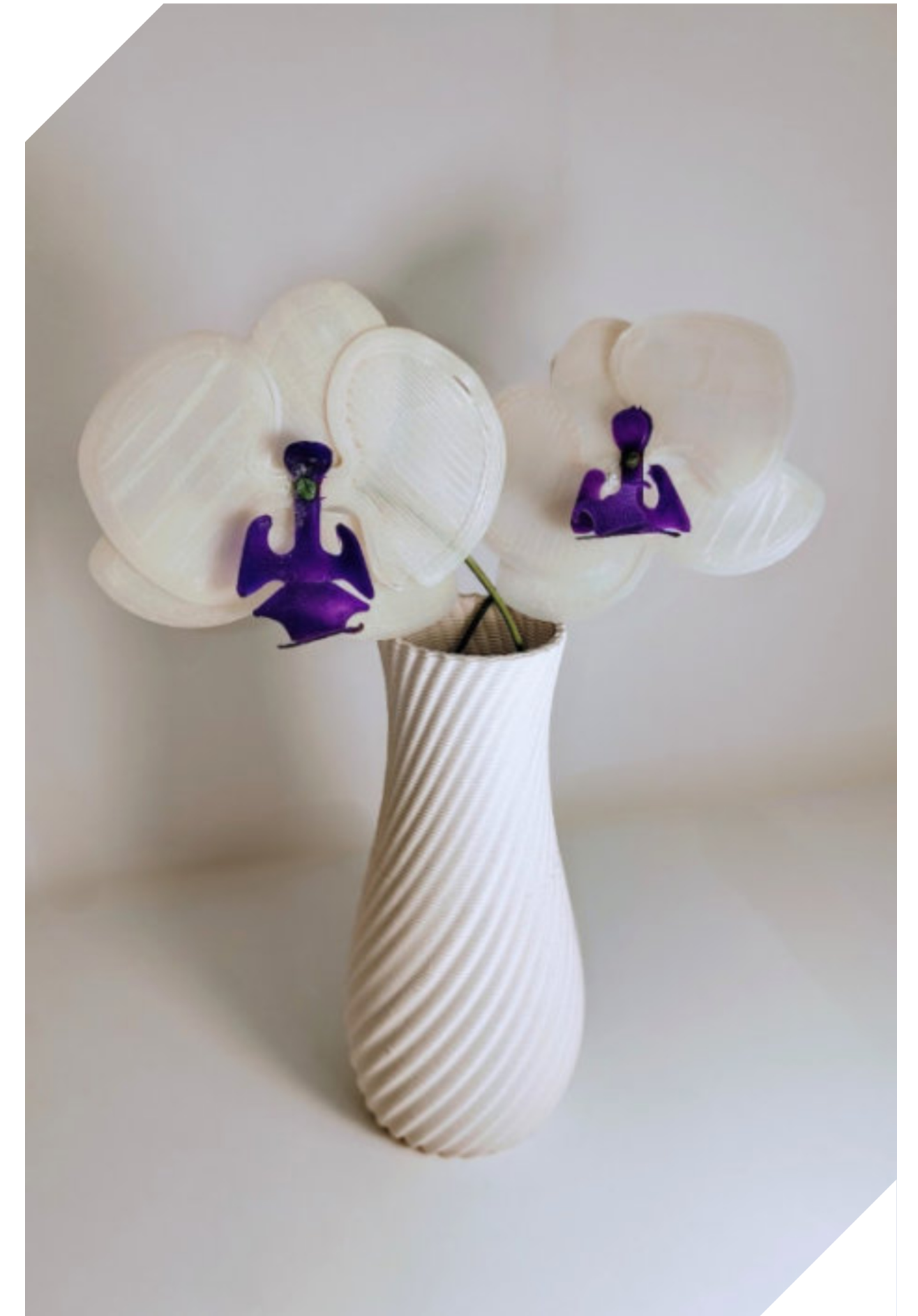
Clay 3D printed vase modelled in the Grasshopper add-on of Rhinoceros
